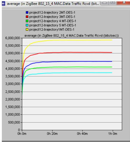
Fig. 11. Data Traffic Received on MT by using different trajectories.
