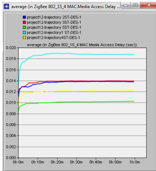
Fig. 13. Media Access Delay of ST by using different trajectories.
