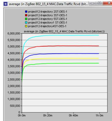
Fig. 10. Data Traffic Received on ST by using different trajectories.
