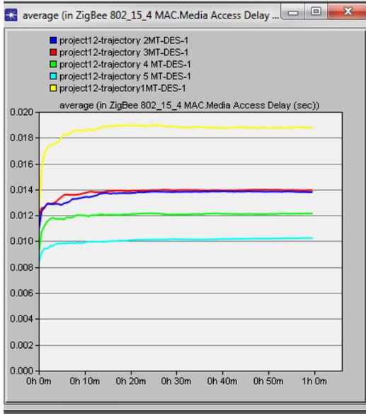
**Fig. 14.** Media Access Delay of MT by using different trajectories.
